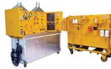
Our HYDRAULIC TEST **STATION** allows us to Pressure Test up to 10,000 PSI
