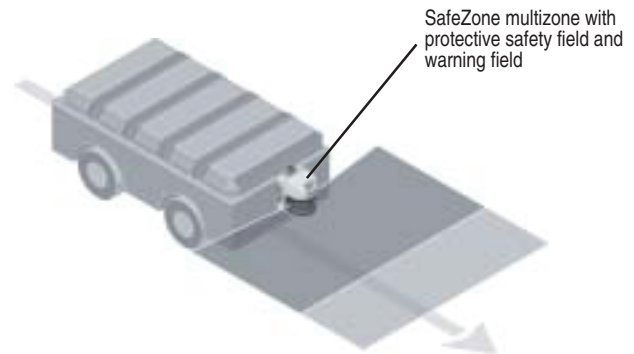
Figure 56: Vehicle monitoring with SafeZone safety laser scanner
