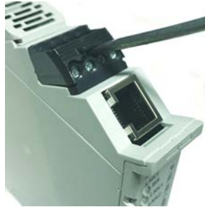
Figure 3 - Terminal Block Removal
