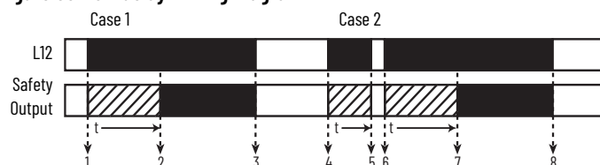
Figure 35 - On-delay Timing Diagram
