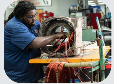
Full Motor Rebuilds / Rewinds
