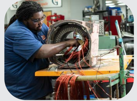
Full Motor Rebuilds / Rewinds
