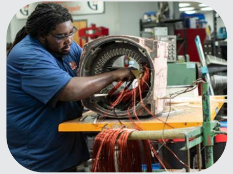
Full Motor Rebuilds / Rewinds
