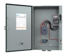
Pump control panel, NEMA Size 4, Three phase full voltage, 150A motor circuit protector, Solid-state overload relay, OLR amp range 50-200A, 480 V AC 60Hz coil, HOA selector switch, Start push button, Enclosure NEMA type 3R, Weather proof outdoor use, Standards: UL 60947-1, Certifications: cULus, Listed Service Entrance Equip
