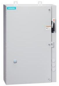
Non-reversing motor starter, Size 2, Three phase full voltage, Solid-state overload relay, OLRelay amp range 13-52a, 220 240/440 480VAC 60HZ coil, Combination type, 60Amp non-fused disconnect Encl NEMA type 4X 304 S-steel Water/dust tight noncorrosive, Extrawide enclosure
