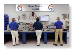
During the repair process, wave form diagnostics are used, as well as test equipment, to ensure your servo motor is functioning within factory specifications. Each servo motor goes through a step by step repair process.
