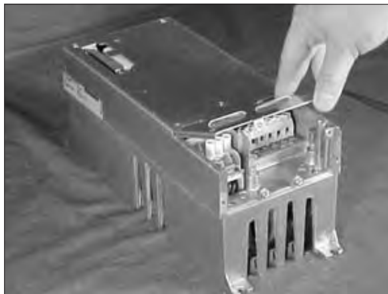
Figure 3-3: Ground Terminal Locations
