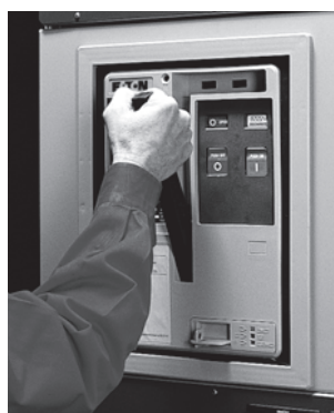
Through-the-Door Design for Human Interface with the Breaker Interface with the Breaker Compartment Door Closed, for Example, Manually Charging the Stored Energy Springs
