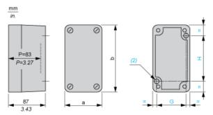
(2)  $2 \times \emptyset$  5.6 mm/0.22 in. holes, depth 12 mm/0.47 in. P Usable depth
