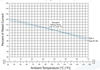
When the temperature difference between the motor and controller does not exceed +10 °C the heater elements should be selected according to the directions given in the Heater Element Selection, page 2.
